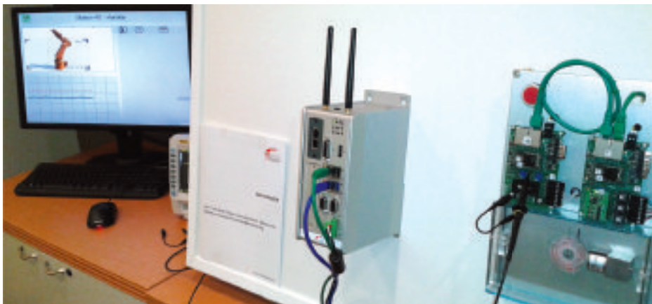
A Hilscher demonstration showed vibration monitoring for drives, with strain gauges, and transfer of data from the edge into the cloud and analytic services. Hilscher plans to be the enabler of field data in Industrial Internet-based architectures. Courtesy: Mark T. Hoske, Control Engineering , CFE Media
